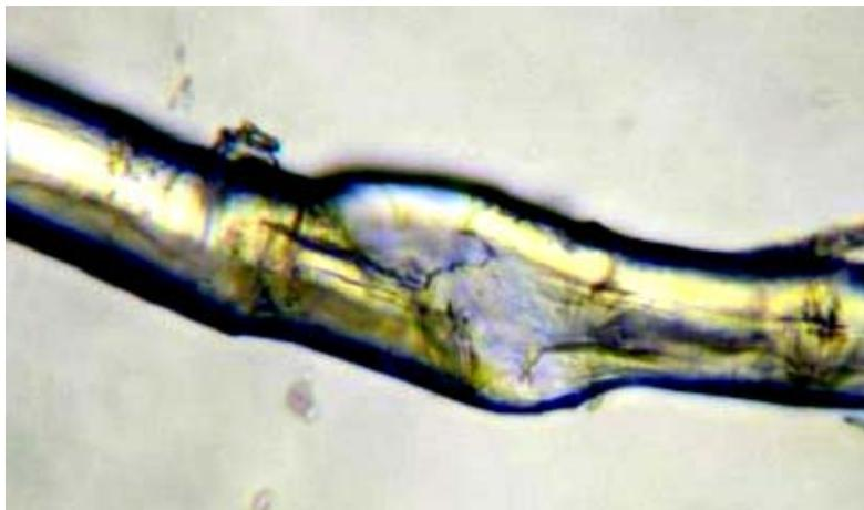
**Figure 9** Microscope view of a single fiber of linen colored after excimer laser irradiation at  $\lambda = 193$  nm. The mechanical damage in the middle shows a colorless medulla, suggesting the color penetrates only the primary cell wall of the fiber, which is about  $0.2 \mu\text{m}$  thick. The fiber has an average diameter of  $20 \mu\text{m}$ .
