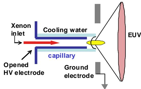
**Figure 5.** Schematic of the DPP shown in Fig. 4.
