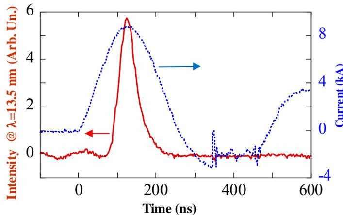
**Figure 7.** Time evolution of the discharge current and of the radiation emission.
