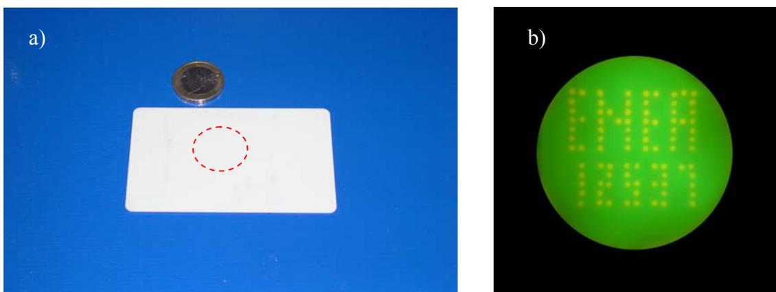
**Figure 8.** a) Picture taken under natural light illumination of a standard plastic card (85 mm×54 mm) with an invisible mark within the dashed area written by the radiation emitted by EGERIA. b) picture of the same dashed area shown in a), but with the pattern made visible by means of the compact and portable ENEA reading system prototype.
