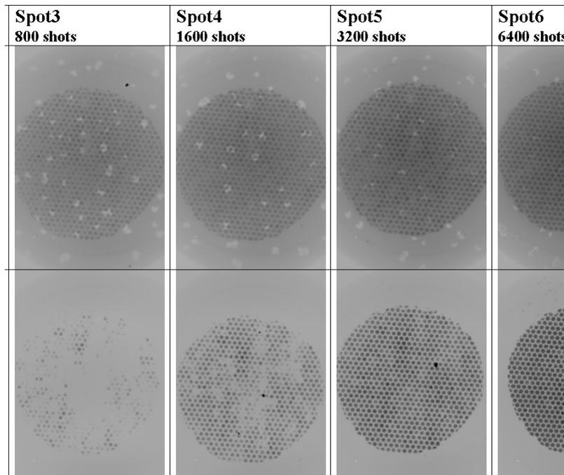
**Figure 3:** Negative photoresists of type “A” (upper row) and of type “B” (lower row), from Birmingham University, exposed to different EUV dose values through a mask having hexagonal holes placed at a distance of 1 mm from the resist. The photoresists are observed under an optical microscope in reflection mode (after development of the resists). The darker regions correspond to higher photoresist thickness.
