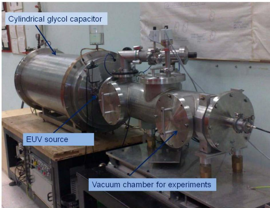
**Figure 4.** Photograph of the DPP operating at the ENEA Frascati Research Centre, with the main components highlighted.
