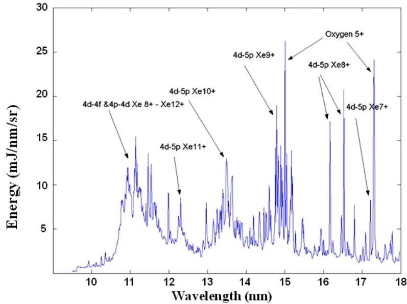
**Figure 6.** Typical spectrum of the radiation emitted by the DPP.
