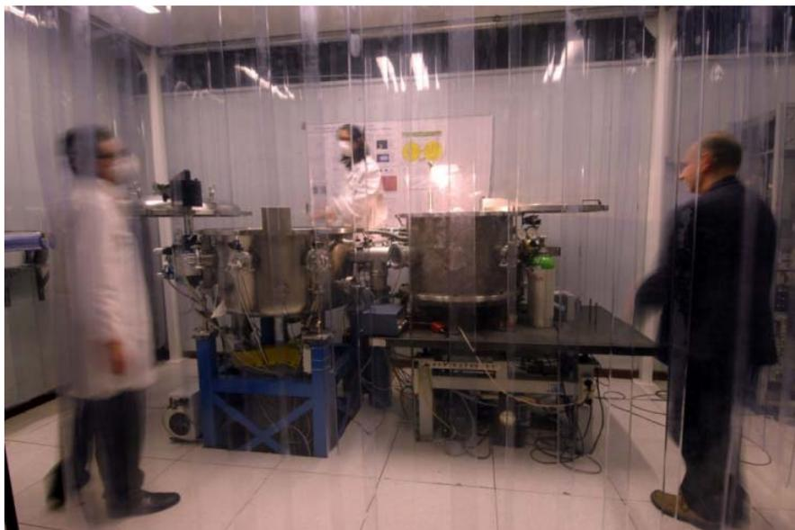
**Figure 2** The EGERIA source (on the right) and the Micro Exposure Tool (on the left) inside the clean room ISO 7 (10.000).
