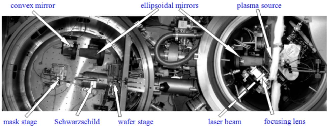
**Figure 1** Top picture of the EGERIA vacuum chamber (right) where the laser-plasma is generated and of the Micro Exposure Tool high-vacuum chamber (left) where sub-micrometer pattern are written either on a photoresist or on a fluorescent material.
