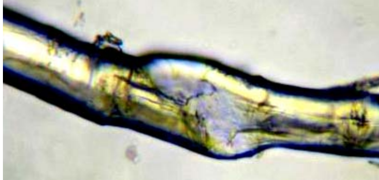
Figure 7. Microscope image of a single linen fiber colored after ArF laser irradiation. The mechanical damage in the central part shows small pieces of colored primary cell wall on a colorless inner part of the fiber. The average diameter of the fiber is 20 \mu\text{m} .
