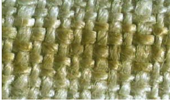
Figure 3. Micro-photographs of the cloth irradiated with 100 XeCl laser pulses. Intensity (fluence) on linen 16 \text{ MW/cm}^2 ( 0.5 \text{ J/cm}^2 ) per pulse.
