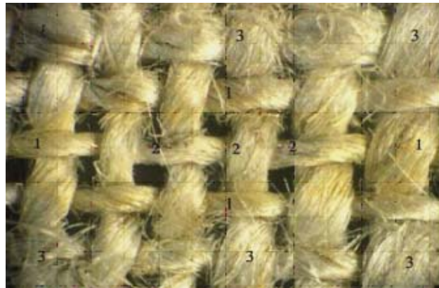
Figure 5. The area of the linen irradiated by the ArF laser beam shows different characteristics that depend on the local values of F(x,y) . 1) colored area; 2) ablated area; 3) area irradiated below the threshold for coloration.
