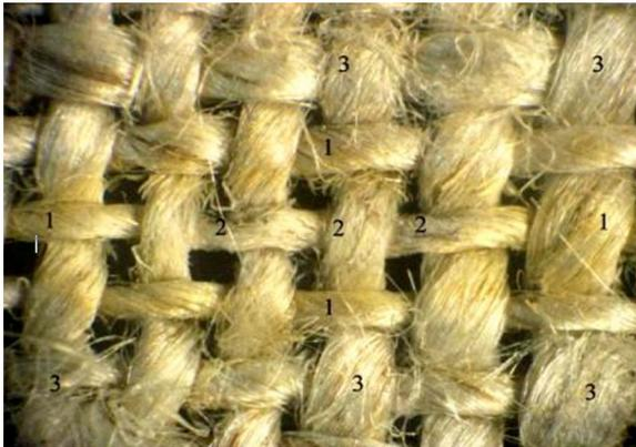
**Figure 5.** Linien area irradiated by ArF laser pulses having different characteristics corresponding to the local laser intensity value  $I(x, y)$ . (1) Colored area. (2) Ablated area where fibers are first colored and then vaporized. (3) Area irradiated below threshold for coloration.
