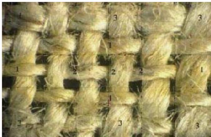
**Figure 5.** The area of the linen irradiated by the ArF laser beam shows different characteristics that depend on the local values of  $F(x,y)$ . 1) colored area; 2) ablated area; 3) area irradiated below the threshold for coloration.
