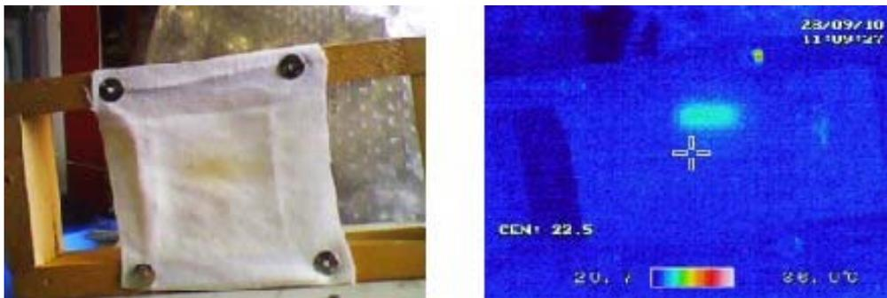
*Figure 13b. Left: photo of the linen during ArF laser irradiation. Right: the same frame seen in infrared light. The color scale reveals that the warmest area of the irradiated linen is at 25  $^{\circ}\text{C}$ , while the non-irradiated area is at the room temperature of 21  $^{\circ}\text{C}$ .*
