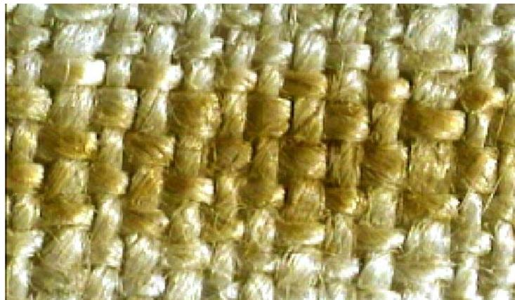
**Figure 3.** *Micro-photographs of the cloth irradiated with 100 XeCl laser pulses. Intensity (fluence) = 16 MW/cm<sup>2</sup> (0.5 J/cm<sup>2</sup>) per pulse.*
