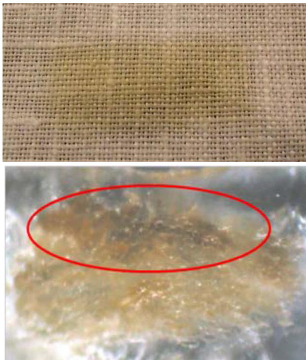
Figure 1. Above: faint linen coloration after 10 laser shots at 308-nm. Fluence/shot 0.15 J/cm 2 . Intensity/shot 4.5 MW/cm 2 . 1 Hz repetition rate. Source: ENEA. Below: cross section of a linen yarn irradiated at 308 nm, contrast enhanced. The red ellipse shows the depth of the coloured region. From [10].
